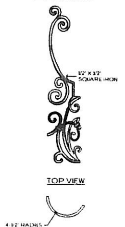
RIGHT TERMINATION LEFT SIDE VIEW
